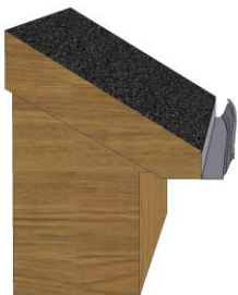
GUTTER LIP RUNNING INTO THE HOUSE
