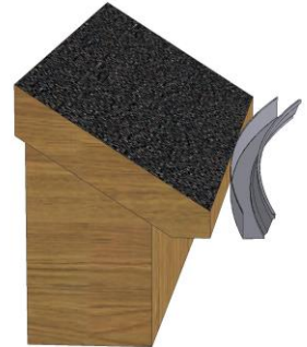
GUTTER RUNNING AWAY FROM THE HOUSE
