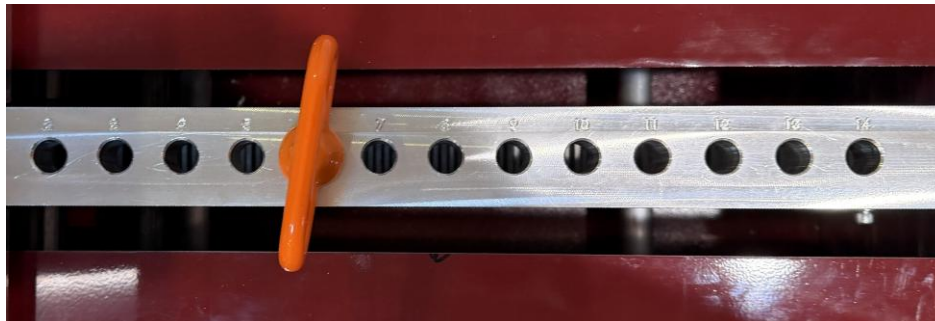
Set the T-handle pin position to control the number of crimps.
