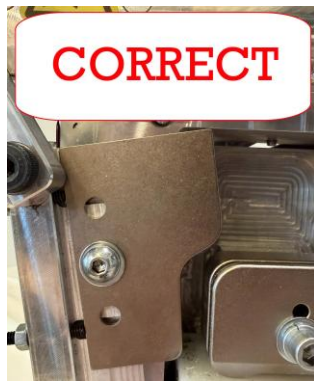
Figure: 10-2: This side of the left knife should face operator when mounted
