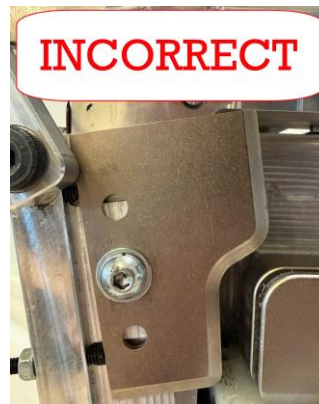
The beveled side of the left knife should face away from the operator when mounted.
