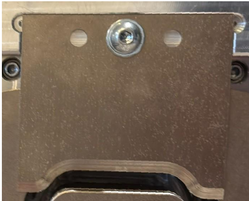
Figure 10-3: This side of the top knife should face the operator when mounted.
