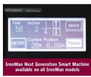
Use the touch screen to automatically control product length, add for miters, if applicable, and keep a total of daily material ran and total footage. Password protected.
