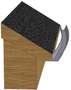
GUTTER RUNNING INTO THE HOUSE
