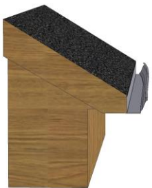
GUTTER LIP RUNNING INTO THE HOUSE
