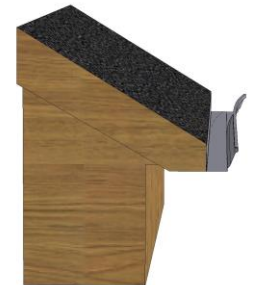
GUTTER LIP RUNNING AWAY FROM THE HOUSE
