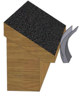
GUTTER RUNNING AWAY FROM THE HOUSE
