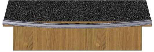
GUTTER RUNNING UPHILL
