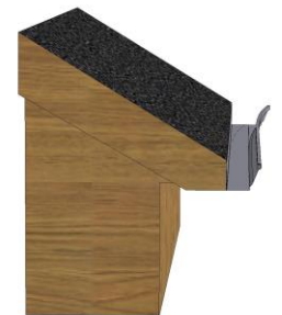
GUTTER LIP RUNNING AWAY FROM THE HOUSE
