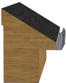
GUTTER LIP RUNNING INTO THE HOUSE
