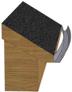
GUTTER RUNNING INTO THE HOUSE
