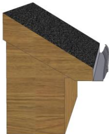
GUTTER LIP RUNNING INTO THE HOUSE
