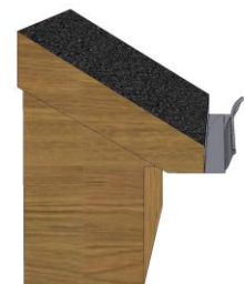
GUTTER LIP RUNNING AWAY FROM THE HOUSE
