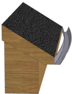
GUTTER RUNNING INTO THE HOUSE
